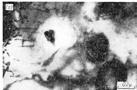
Photo.4 Electron transmission micrograph of spheroidized pearlitic steel (statically 4.0% strained)
