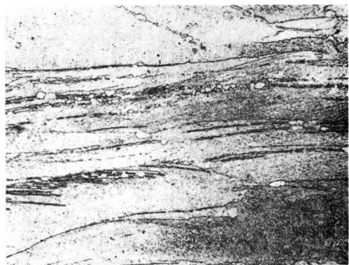
Photo. 4 Metallographs of recrystallization of the dynamically deformed iron. (×100) (a) 600°C×10 min
