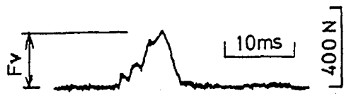
WA80H7V, SKH4, V_s=35\text{m/s} , a=3\text{mm} , V_w=179 \mu\text{m/s} , b=3\text{mm} , 2A=1\text{mm} , Down-cut
