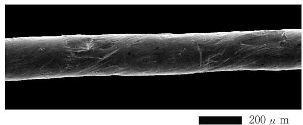
Fig. 13 SEM view of the surface appearance of Sn-9Zn-1mass%Al alloy fiber produced by in-rotating-ethanol-spinning process.
