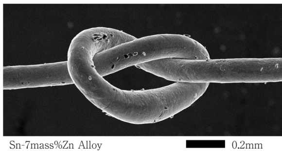
Fig. 6 SEM view of the as-cast Sn-7mass%Zn alloy fiber with full ductility.
